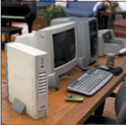
The Back-UPS® RS for high performance power protection (pictured above) offers versatile mounting options: tower, under monitor, and 2U shelf mount.
